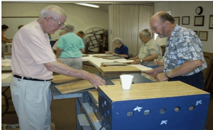
Wayne Galler & Don Weed feed braille plates through a press that embosses the dots on the paper.
